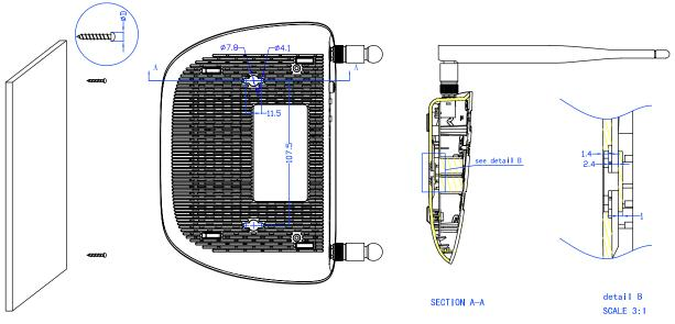
Figure 2-1 Wall-mount Install
