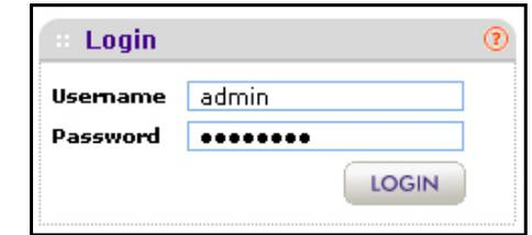
2. Enter **admin** for the user name and **password** for the password, both in lowercase letters. The web management interface of the access point displays. The menu lets you navigate to the various screens.
