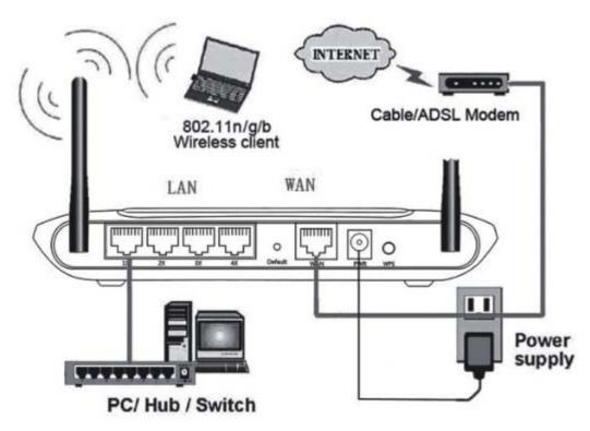
Attach one end of an Ethernet cable to your computer's Ethernet port, and the other end to one of the LAN ports of your router.
