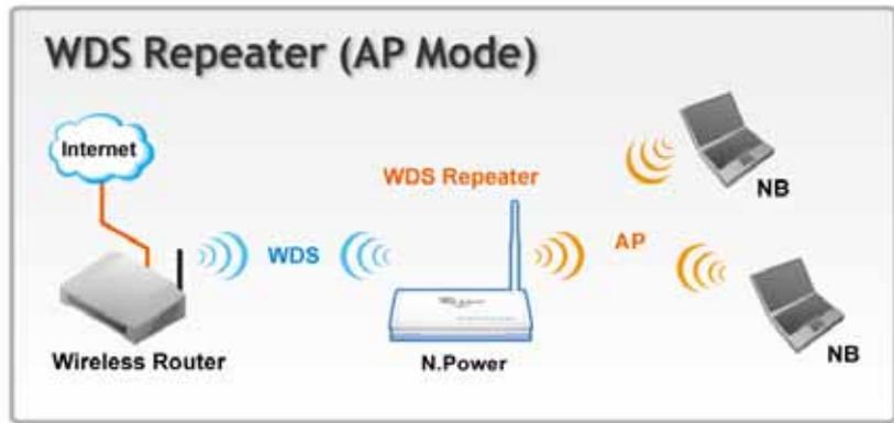
This is known as WDS Repeater function. In AP mode, the N.Power will repeat the wireless signal of remote AP/Router. Up to 4 WDS repeaters can be connect with N.Power. WDS works by entering the wireless MAC addresses (also known as BSSID) of remote Access Points.
