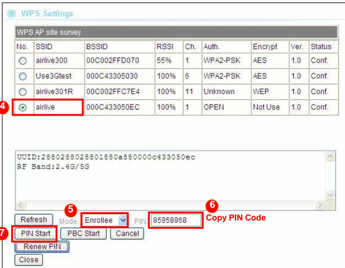
Under AP site, Select Wireless Setting → WPS Setting. Choose WPS mode to “PIN” then enter the PIN Code → click “Apply” and the connection will automatically configure.
