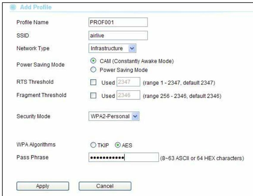
3. Once apply the new profile should appear on the list. Select the profile and click on “Activate” button to take effect. Only one profile can be activated at a time.
