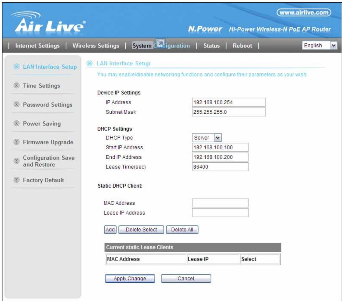
The screenshot displays the Air Live web management interface for an N.Power Hi-Power Wireless-N PoE AP Router. The top navigation bar includes links for Internet Settings, Wireless Settings, System Configuration (selected), Status, and Reboot. A language dropdown menu is set to English. The left sidebar contains a list of configuration options: LAN Interface Setup (selected), Time Settings, Password Settings, Power Saving, Firmware Upgrade, Configuration Save and Restore, and Factory Default.
