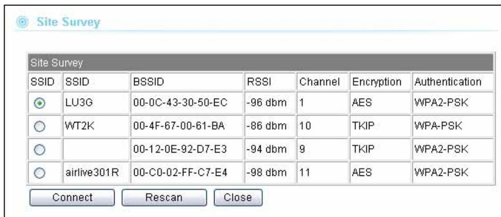
You can now select the SSID you want to connect with, and then press the “Connect” button. If encryption key is required, the AP will prompt you to enter the encryption information.
