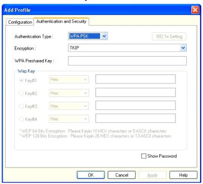
**Authentication Type:** This setting has to be consistent with the wireless networks that the adapter intends to connect.
