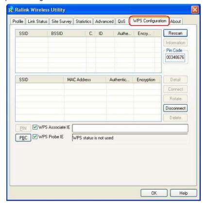
**WPS Site Survey:** Display the information of surrounding APs with WPS IE from last scan result. List information's include SSID, BSSID, Channel, ID (Device Password ID), Authentication Type and Encryption Type.
