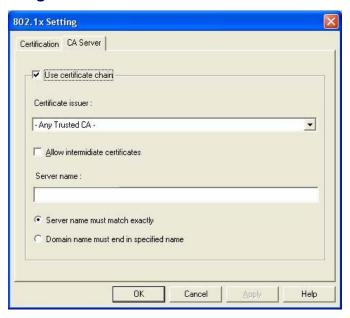
**Use Certificate Chain:** When the EAP authentication types such as TLS, TTLS or PEAP is selected and required a certification to tell the client what server credentials to accept from the authentication server in order to verify the server, you have to enable this function.
