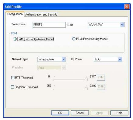
**Profile Name:** Define a recognizable profile name for you to identify the different network.
