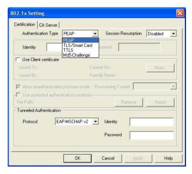
**Authentication Type:** The EAP authentication protocols this adapter has supported are included as follows. This setting has to be consistent with the wireless APs or Routers that the adapter intends to connect.
