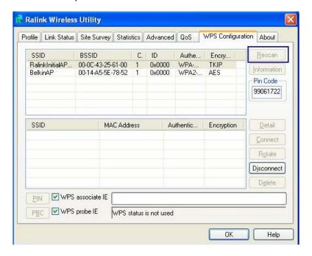
Step2: Select an AP(SSID/BSSID) that STA will join to.
