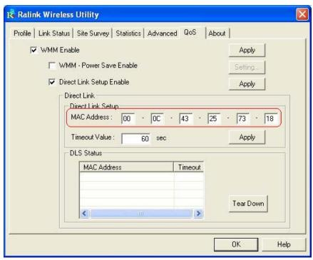
2. Timeout Value represents that it disconnect automatically after some seconds. The value is integer. The integer must be between 0~65535. It represents that it always connects if the value is zero. Default value of Timeout Value is 60 seconds
