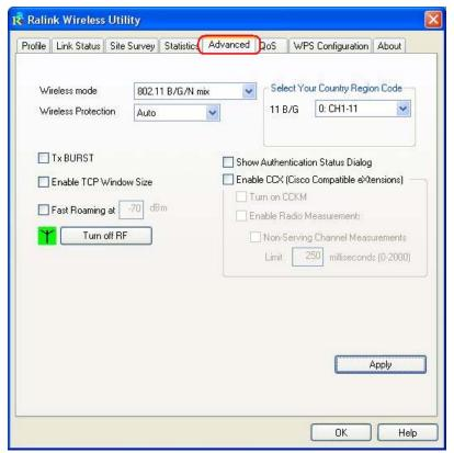
**Wireless Mode:** Select wireless mode. 802.11 B only, 802.11 B/G mix, 802.11 B/G/N mix, 802.11 B/G mix, and 802.11 B/G/N mix modes are supported
