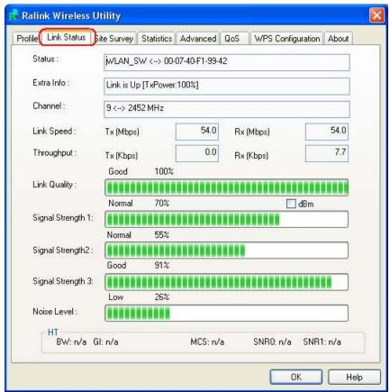
**Status:** Current connection status. If no connection, it will show Disconnected. Otherwise, the SSID and BSSID will show here.
