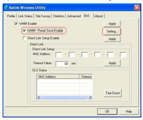
**Step2**: After clicking "**Setting**..." button, show "**Power Save Setting**" dialog. Please select which ACs you want to enable. Then click "**Apply**" button. The setting of enabling WMM – Power Save is successfully.
