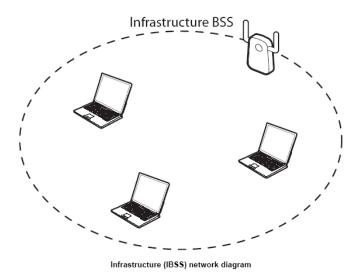
In the ESS diagram below, communication is done through the access points, which relay data packets to other wireless stations or devices connected to the wired network. Wireless stations can then access resources, such as a printer, on the wired network.
