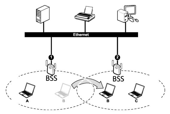
Roaming in an ESS network diagram
