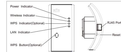
**NOTE:** If you need to **reset** the Wi-Fi Repeater, you need press and hold the reset button inside the tiny hole for **10** seconds.
