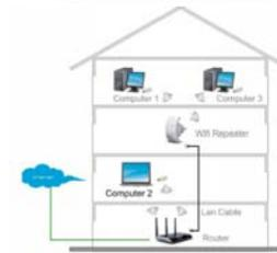
Connect the WiFi-Repeater to your Router/Switch with RJ-45 Cable
