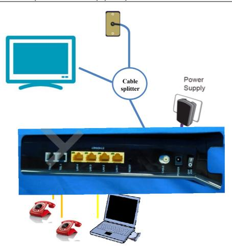
The screen of the coaxial cable is intended to be connected to earth in the building installation
