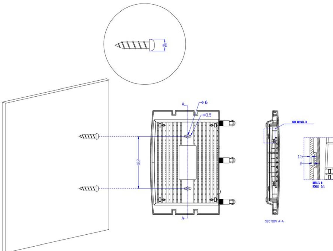
Figure 2-1 Wall-mount install
