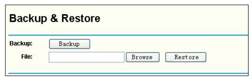
Figure 5-27 Save or Restore the Configuration
