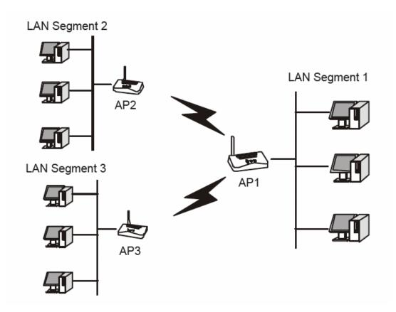
Figure 5-9 Point to Multi-point Bridge
