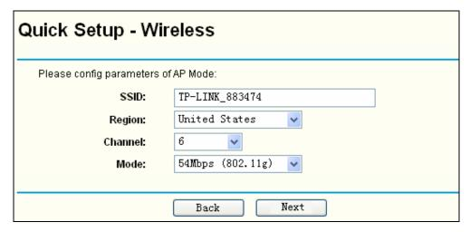
Figure 3-11 Quick Setup - Wireless settings
