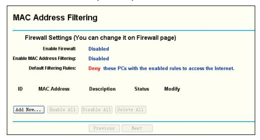
Figure 4-41 MAC address Filtering
