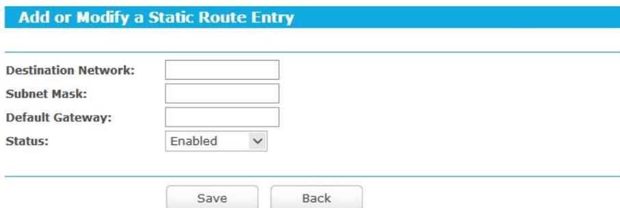
Figure 5-75 Add or Modify a Static Route Entry
