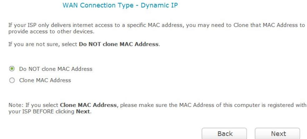
Figure 3-6 Quick Setup – MAC Clone
