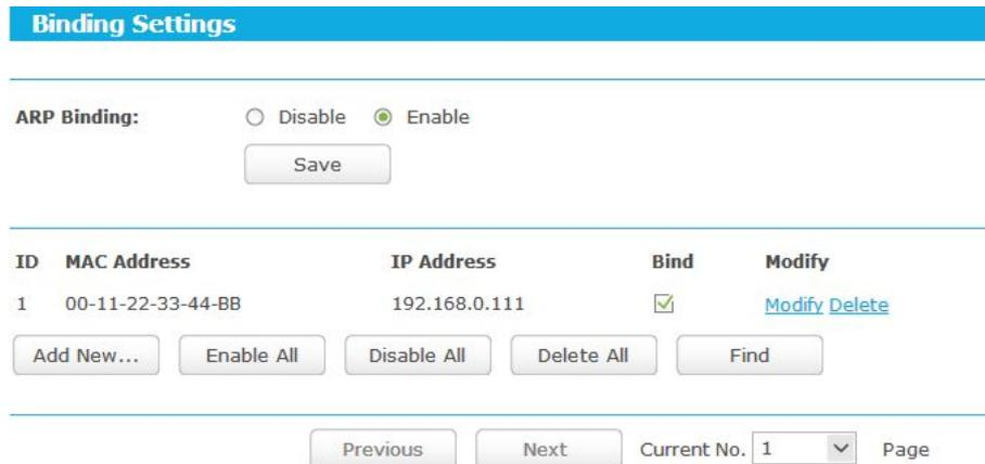
Figure 5- 80 Binding Setting
