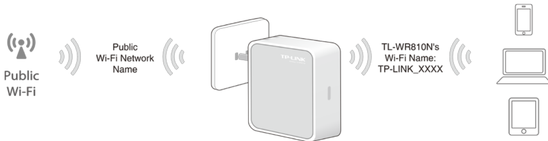
Figure 2-5 Hardware Installation of the TL-WR810N in Hotspot Router Mode
