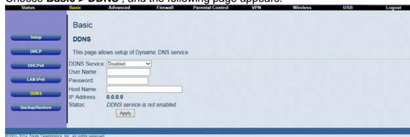
Figure 14 DDNS setup
