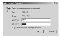
If you are not prompted for a **User Name** and **Password**, do the following in this order: Recheck all connections; restart the modem and computer; and reset the modem by inserting a paper clip into the **Reset** pinhole in the modem's back panel and press it three times.
