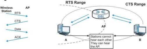
When station **A** sends data to the AP, it might not know that the station **B** is already using the channel. If these two stations send data at the same time, collisions may occur when both sets of data arrive at the AP at the same time, resulting in a loss of messages for both stations.
