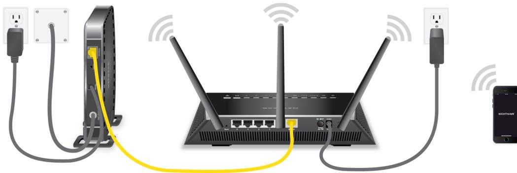
Figure 5. Router cabling
