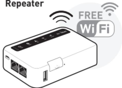
Using **Repeater** means connecting your mini router to another existing wireless network, e.g. when you are using Wi-Fi in hotels or other public locations.
