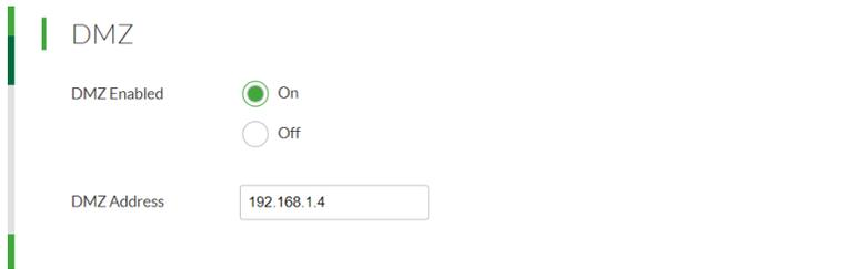
6. Select the DMZ Enabled **On** radio button.
