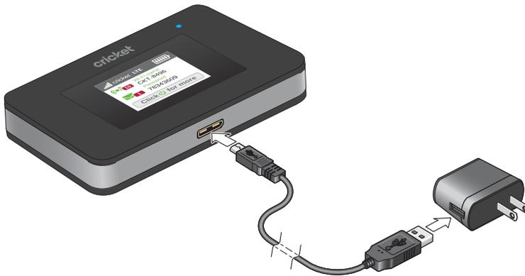
2. Connect the other end of the cable to the USB port on your computer or to the USB charger.
