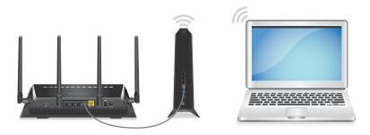
Figure 4. Extender in access point mode
