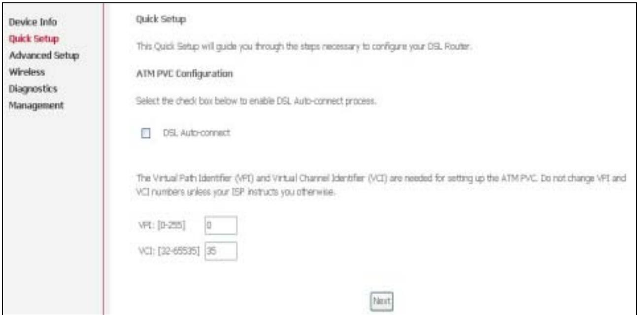
Figure 11. Quick Setup – ATM PVC Configuration
