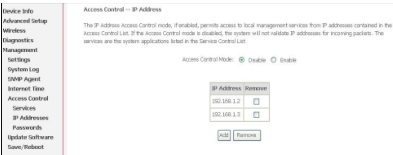
Figure 68. Management – Access Control – IP Addresses
