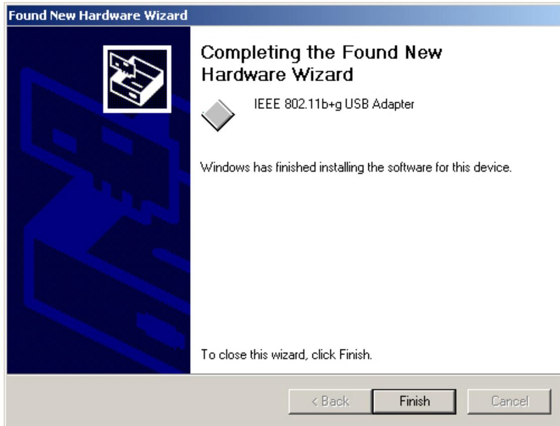
After finishing the phase 1 installation of the driver, the NoteBook (or PC) with WinME OS shall be restarted, but Win2000 or WinXP OS doesn't need to be restarted.
