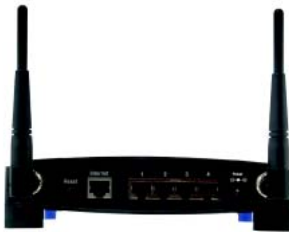
Figure 3-1: The Broadband Router's Back Panel
