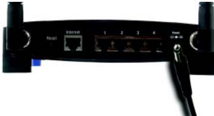
Figure 4-3: Connecting the Power
