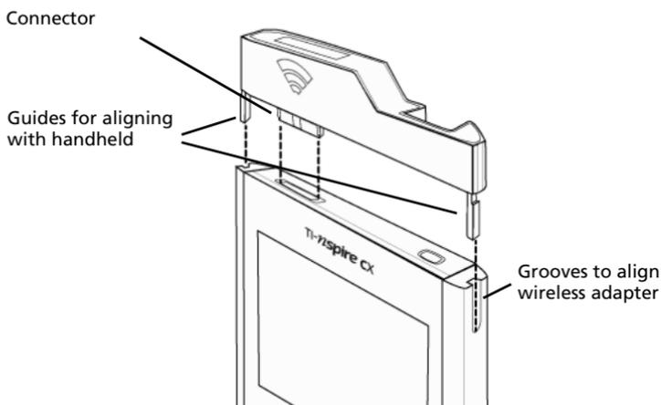
2. Slide the adapter into position, making sure the guides on the sides of the adapter slide into the grooves on the sides of the handheld.
