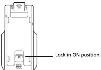
5. Insert each cradle into the charging bay. Make sure the LED is amber.
