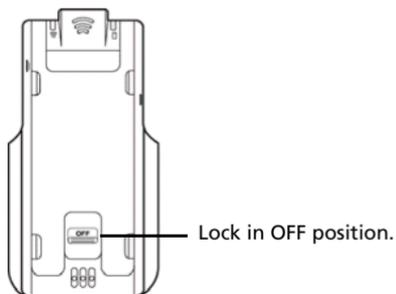
2. To attach the handheld, face the screen upward and slide the handheld onto the top of the TI-Nspire™ Navigator™ wireless cradle. Be sure that both sides of the handheld are inserted into both of the side guides.
