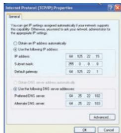
5. If "Use the following IP address" (2) is selected, your Router will need to be set up for a static IP connection type. Write the address information in the table below. You will need to enter this information into the Router.
