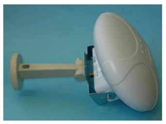
Figure 9. Exciter attached to the flexible mount.
