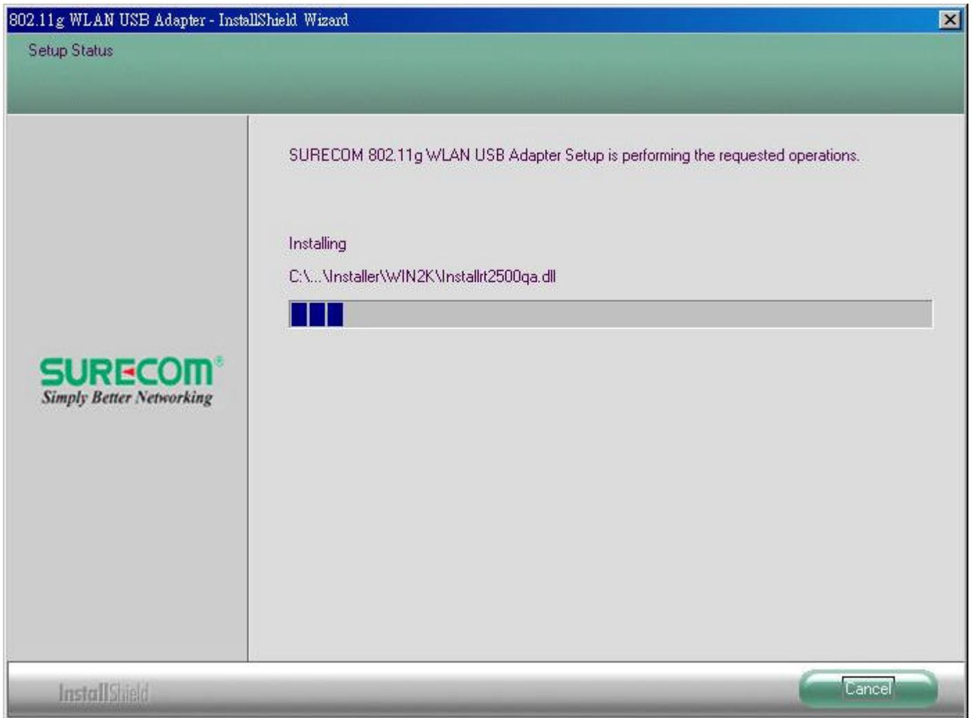
Plug-in the WLAN USB Adapter into your USB slot when the window below appears.
