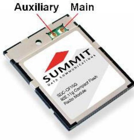
*The SDC-CF10G module has two connectors for 2.4 GHz antennas.*
