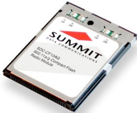
*The SDC-CF10AG module has two connectors for 2.4 GHz antennas and two connectors for 5 GHz antennas.*
