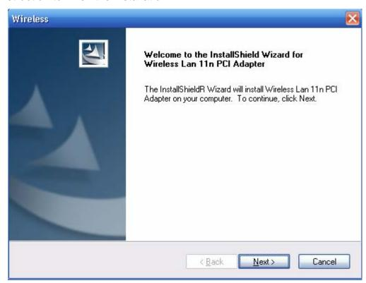
After complete the procedure, insert your WLAN card into PCI connector of your system, and then system will detect new hardware. Select "Install the software automatically (Recommended)", and then click **Next** to continue. After copy the file to your system, then the setup is finish.
