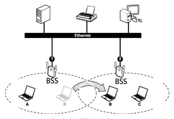
Roaming in an ESS network diagram
