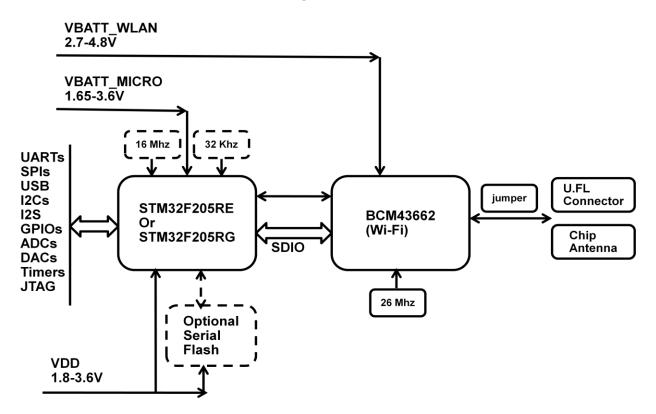
RZ707MS Module consists of two main components: an ARM Cortex-M3 based 32-bit microcontroller that runs Em-Fi Software and Broadcom BCM43662 Wi-Fi device. It also includes an optional serial Flash (1MB or 2MB), an on-board chip antenna and a u.FL connector for optional external antenna.
