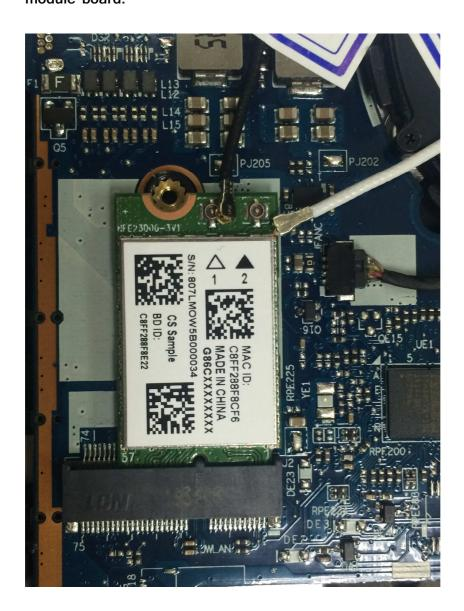
Step 3. Remove the Wireless PCle NGFF1630 module board from PCle
