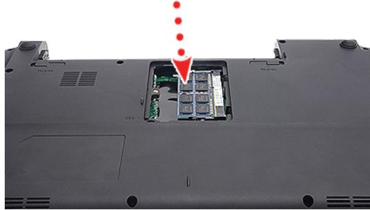
4. After inserting the memory, fasten the cover with the screws.
