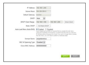
is no connection available, the Repeater will act as a DHCP Server. You may also manually control the IP settings of the Dual Band Repeater by choosing Client, Server or Disabled from the DHCP drop down menu. This is only for advanced users.
