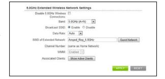
Broadcast SSID: Selecting Disable Broadcast SSID will hide the visibility of the repeater's SSID. Users must manually enter the SSID to connect.
