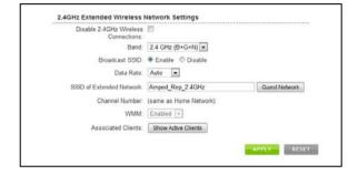
Broadcast SSID: Selecting Disable Broadcast SSID will hide the visibility of the repeater's SSID. Users must manually enter the SSID to connect.
