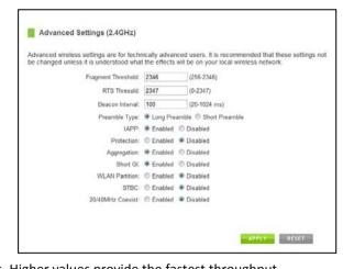
Beacon Interval: Indicates the frequency interval of the beacon. A beacon is a packet broadcast by the repeater to sync the wireless network.
