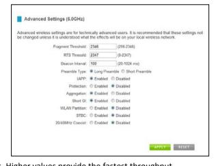
Beacon Interval: Indicates the frequency interval of the beacon. A beacon is a packet broadcast by the repeater to sync the wireless network.
