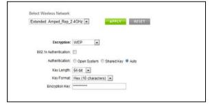
Using the drop down menu, you can select which network you wish to configure and may adjust the security settings below.
