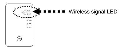
(5) Please move this Range Extender to the place you wish to use (a better place will be the center of your house) and insert this Range Extender into power outlet on the wall, the wireless connection will be established automatically.
