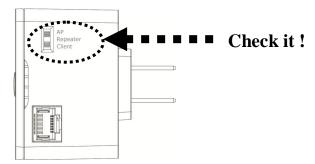
This Range Extender supports AP, Repeater and Client modes, The default mode is "Repeater mode", you can also switch it to another mode while you're using this Range Extender
