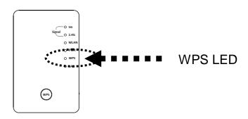
When connection is created, the 5G or 2.4G signal LED will turn on.
