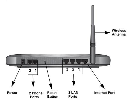
Figure 1-2: wireless router Rear Panel
