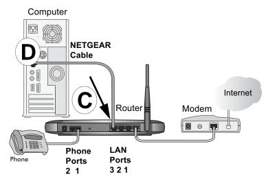
Figure 3-3: Connect the computer to the wireless router
