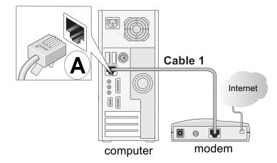
Figure 3-1: Disconnect the Ethernet cable from the computer
