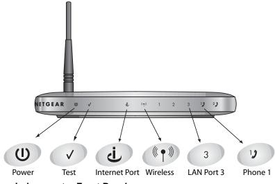
Figure 2-1: wireless router Front Panel
