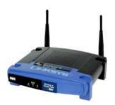
Setup Access Point on the area which MS-6874 RF reachable, and turn on the DHCP function without encryption.
