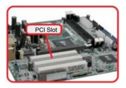
**Step 2.** Put the PC54AG (MS-6845) directly over the PCI slot and press it into the slot firmly.
