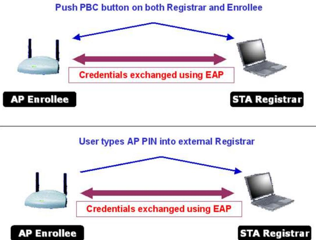
Select an AP (SSID/BSSID) that STA will config and Select the “PIN/numeric code” method.
