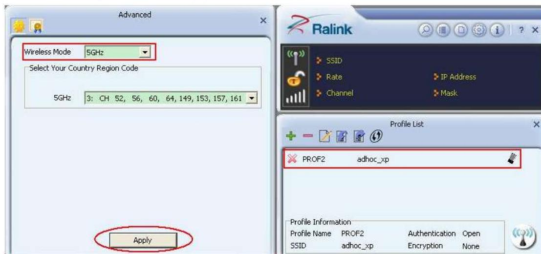
Figure 5-1 Switch wireless mode when activate an adhoc profile
