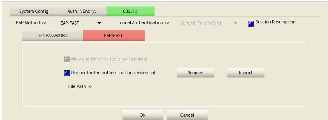
**Allow unauthenticated provision mode:** Mark to enable unauthenticated provision mode.
