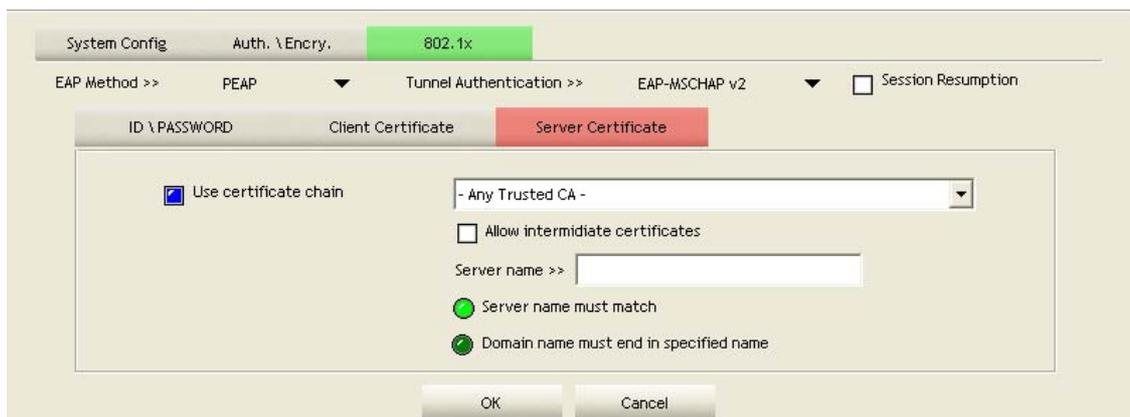
**Use Certificate chain:** Mark the checkbox to enable using certification chain.
