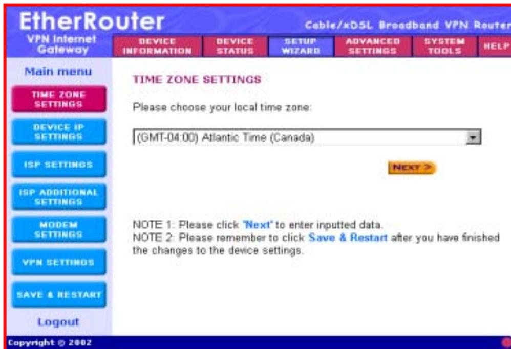
The Setup wizard will take you through 7 step-by-step (7 steps: buttons on the left) configuration procedures that you'll need to do in order to setup the Internet Gateway (e.g. connecting to the Internet / establishing a VPN connection).
