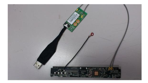
WiFi module connects with USB connector through 6-pin connector, and US connector connects to system to acquire power to operate WiFi module. WiFi module connects with sensor board through 2pcs 26 cm RF cable.
