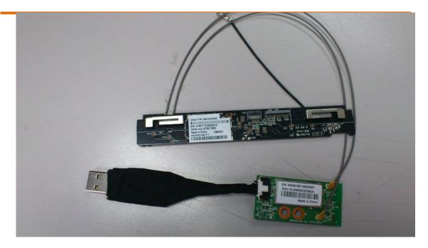
WiFi module uses 2 metal antennas on sensor board as its antennas to transmit and receive data.
