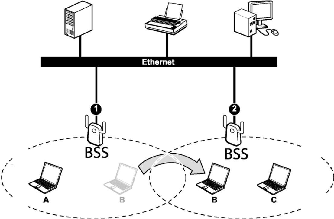
Roaming in an ESS network diagram
