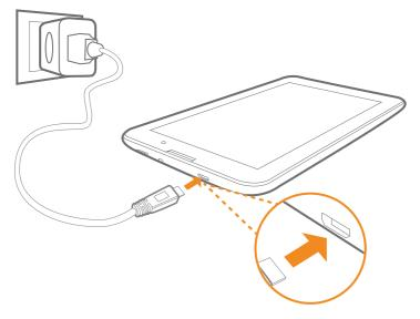
When the battery level falls below the threshold, IdeaTab will alert you with a tone and the battery status icon will change into **I**. We recommend you plug the AC power adapter into your IdeaTab in the direction of the orange arrow as shown above figure.
