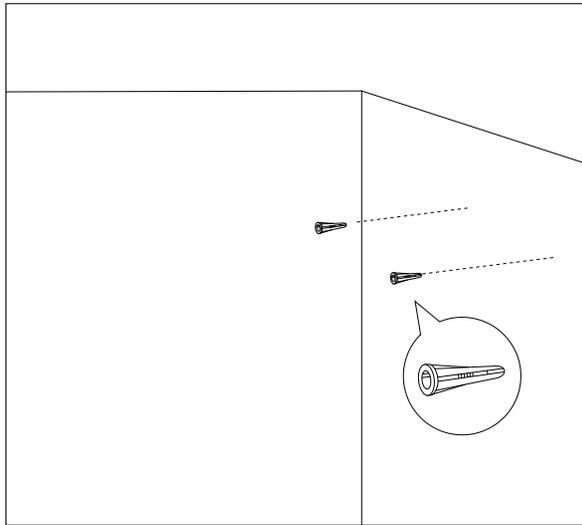
B. Drive the two provided screws into the screw anchors in the wall or partition where the device is to be placed.
