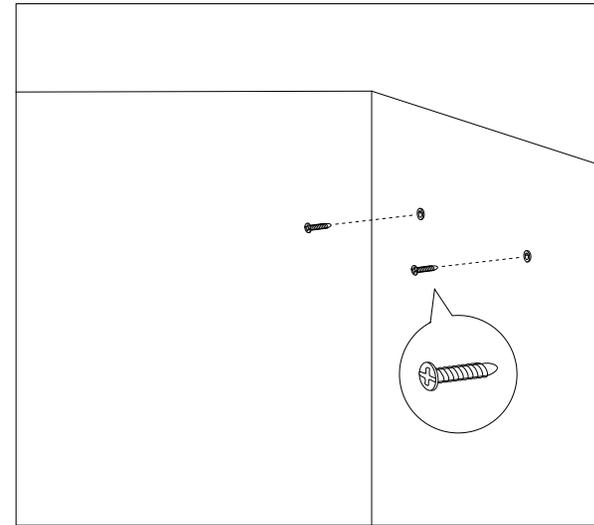
C. Place the mounting holes on the bottom of the device over the screws to mount it to the wall or partition.
