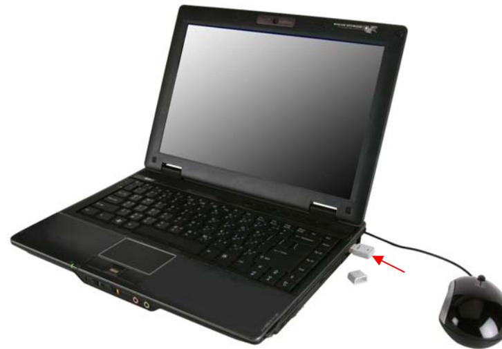
8. The **Found New Hardware** icon will display in the Windows Taskbar. The Found New Hardware Wizard will automatically install the driver for the Wireless N 150 USB adapter.
