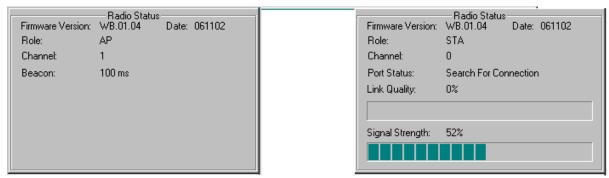
Figure 3. Radio Status Panels (AP: left; Station: right)
