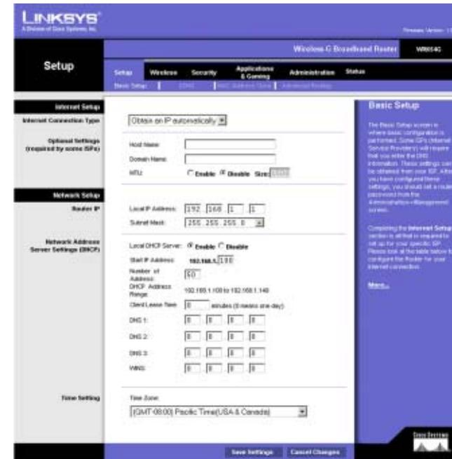
Figure 5-2: Setup Tab - Basic Setup
