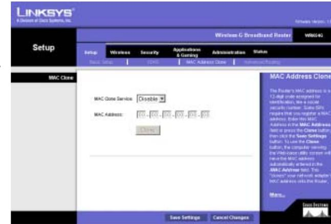
Figure 5-15: Setup Tab - MAC Address Clone
