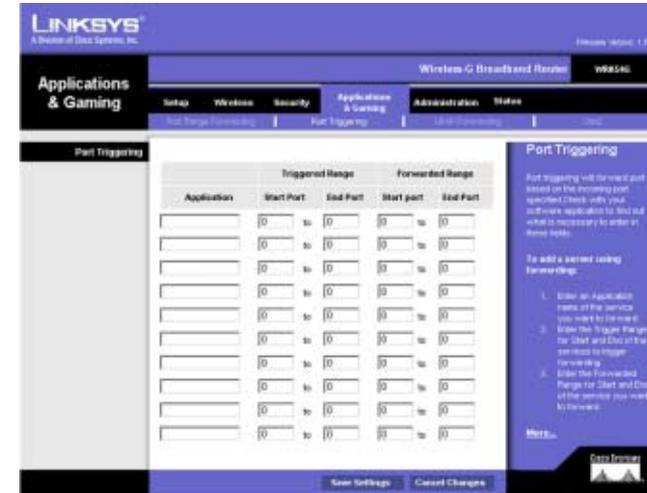
Figure 5-29: Applications and Gaming Tab - Port Triggering
