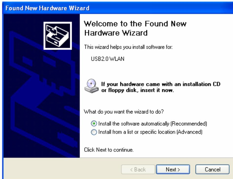
2.4 Your PC will recognize the device of “802.11g USB 2.0 WLAN Adapter”, and click “Next” to install driver.
