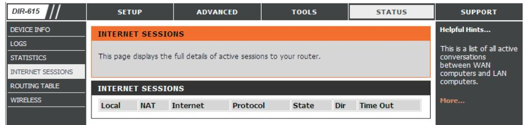
**Time Out:** The number of seconds of idle time until the router considers the session terminated. The initial value of Time Out depends on the type and state of the connection.
