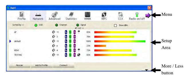
RaUI consists two parts: Menu and setup area. You can select a setup function (Profile, Network, etc.) from menu, and corresponding setup items will be displayed at setup area.
